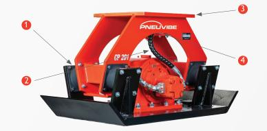
PneuVibes patented system ensures increased elastomer life and minimises vibration transmitted to the boom, thus reducing wear on the pins and bushes of the excavator. Rubber vibration mounts are angled to the base so that the pressure exerted by the boom on the top plate causes the mounts to convert from a shear to a compression mode.
