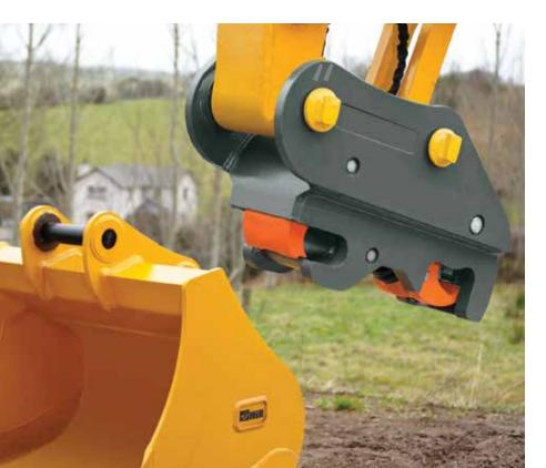
An award-winning quick hitch offers a simple comprehensive solution which uses a positive locking system rather than a gravity locking system thus making this crucial safety feature 'active' and not 'passive'.
