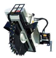
Simex Trenching Wheels are ideal for small fixed-section trenching i.e. for the laying of utilities up to a maximum depth of 800mm and width of 30-250mm on asphalt, concrete and rock.
