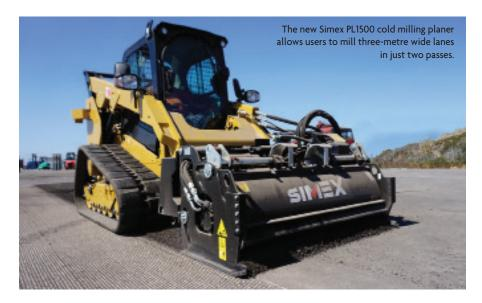
esigned for milling deteriorated surfaces for resurfacing, the Simex PL1500 is an essential tool for today's milling and construction industries.
