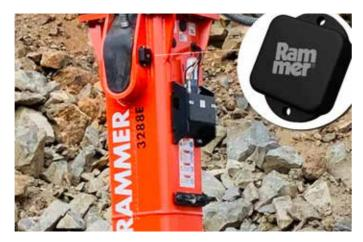
simply log into the MyFleet platform to see all the data on operating hours, how the rockbreaker is being operated and required service intervals helping them manage service periods and minimize machinery downtime by scheduling maintenance during times of least impact on production," Scurr added.
