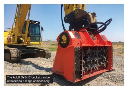
bucket. Current applications include construction waste, composts, glass, soil, manure, and even high moisture material.
