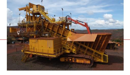
the maximum and minimum limits of the boom reach. This allows the boom to work with its hydraulic cylinders near mid-stroke, allowing for hydraulic cushioning of the hydraulic cylinders and proper operation of hydraulic relief valves, which are used to limit undue stresses on the boom.
