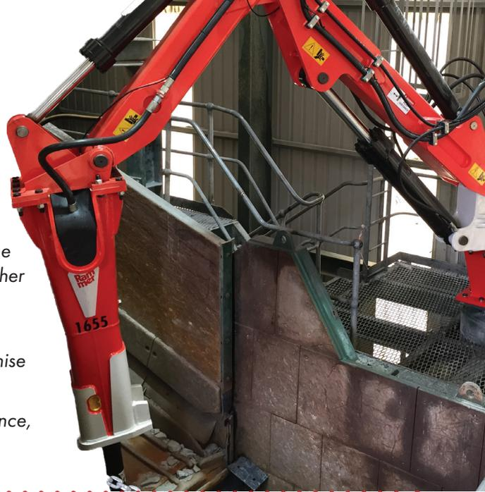
Pedestal mounted hydraulic boom systems are typically installed above crusher inlets or ROM hoppers and grizzly screens to minimise downtime and avoid damage caused by oversize product blocking chutes or crusher inlets.
